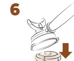
**Empty and clean the portafilter with a cloth that does not damage it**
