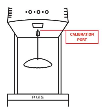
3 With ceramic burrs installed, burr contact is indicated by a change in motor pitch.
