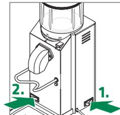
Switch on main switch, also press the grinding button
