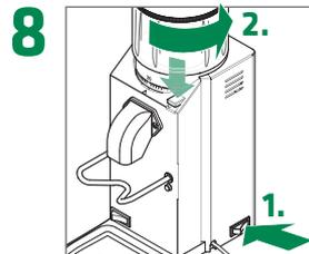
8 If the grinder blades touch, immediately turn off the grinder and turn the bean hopper 2 to 3 notches
