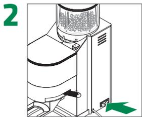
2 Grind requested amount of coffee, then switch off the main switch
