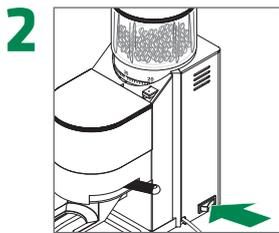
Switch on main switch, grind the coffee beans and switch the main switch off
