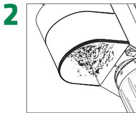
Remove the ground coffee from the ground coffee chamber
