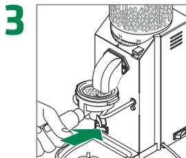
3 Keep the grinding button pressed until you reach the desired amount
