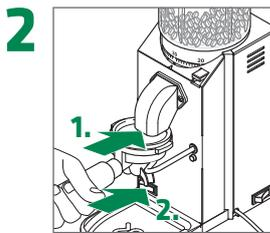
2 Insert filter holder and use the grinding button to grind the coffee directly into the filter holder
