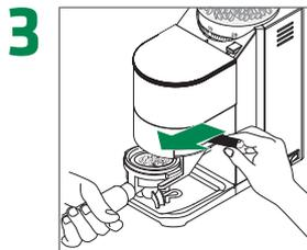
Place the filter holder on the fork and move the dosage lever to release the portion of ground coffee
