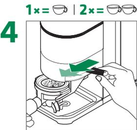
4 Fill the coffee into the filter holder by using the dosage lever
